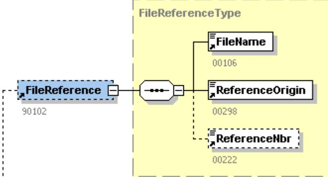
The diagram illustrates the structure of the **FileReferenceType** element. It consists of a central **FileReference** element (90102) connected via an association to a **FileReferenceType** element. The **FileReferenceType** element contains three fields: **FileName** (00106), **ReferenceOrigin** (00298), and **ReferenceNbr** (00222).
